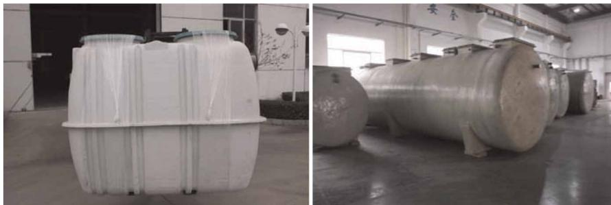
**Figure 2** | Low-power prefabricated wastewater treatment equipment in China.
