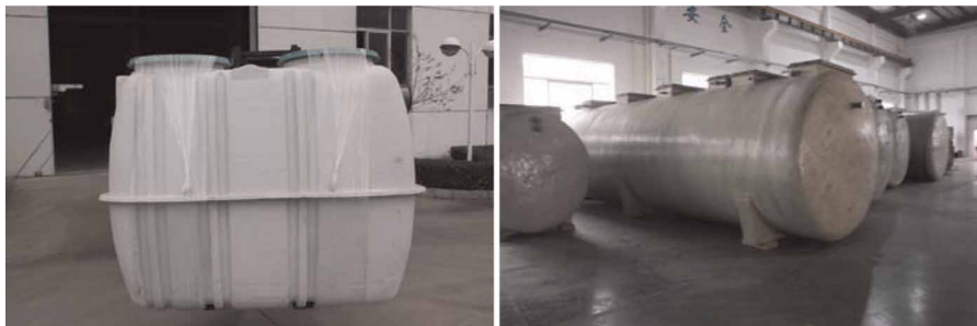
Figure 2 | Low-power prefabricated wastewater treatment equipment in China.
