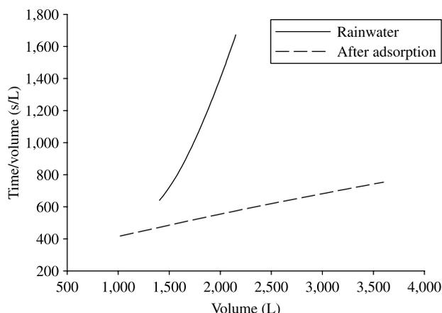
**Figure 6** | Time (s)/permeate volume (L) vs permeate volume (L) after PAC adsorption (pressure = 2 bar; temperature = 25°C; diameter of membrane used = 47 mm).
