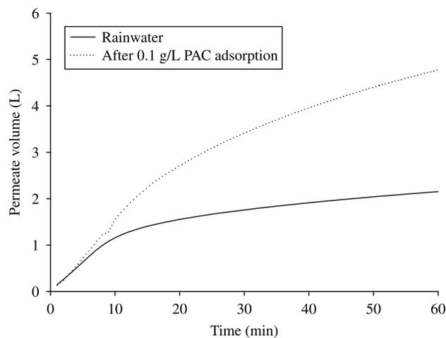
Figure 5 | Time vs permeate volume after PAC adsorption (pressure = 2 bar; temperature = 25°C; diameter of membrane used = 47 mm).
