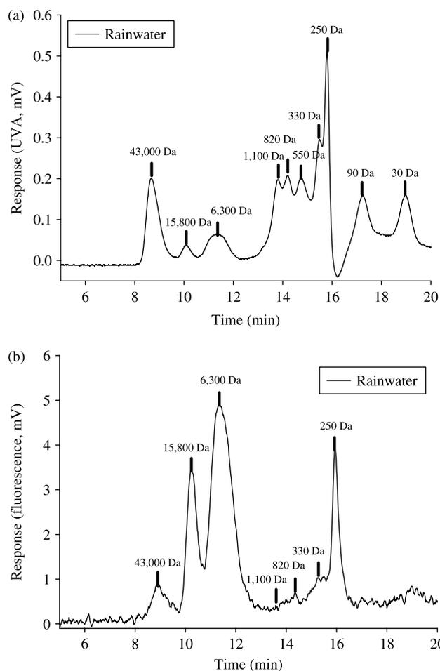
**Figure 2** | MWD of organic matter in rainwater in terms of (a) UV and (b) fluorescence responses.
