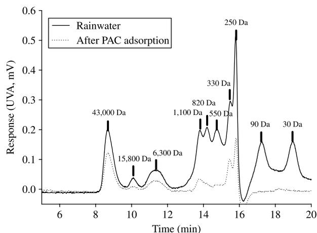
Figure 4 | MWD of organic matter after 0.1 g/L PAC adsorption in rainwater.
