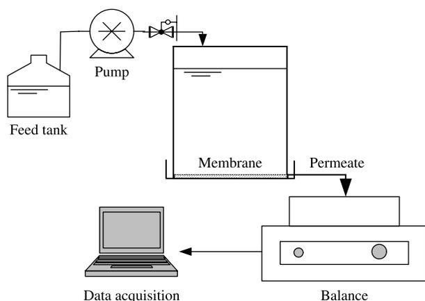
**Figure 1** | Schematic diagram of dead-end cell unit for membrane fouling index experiment.
