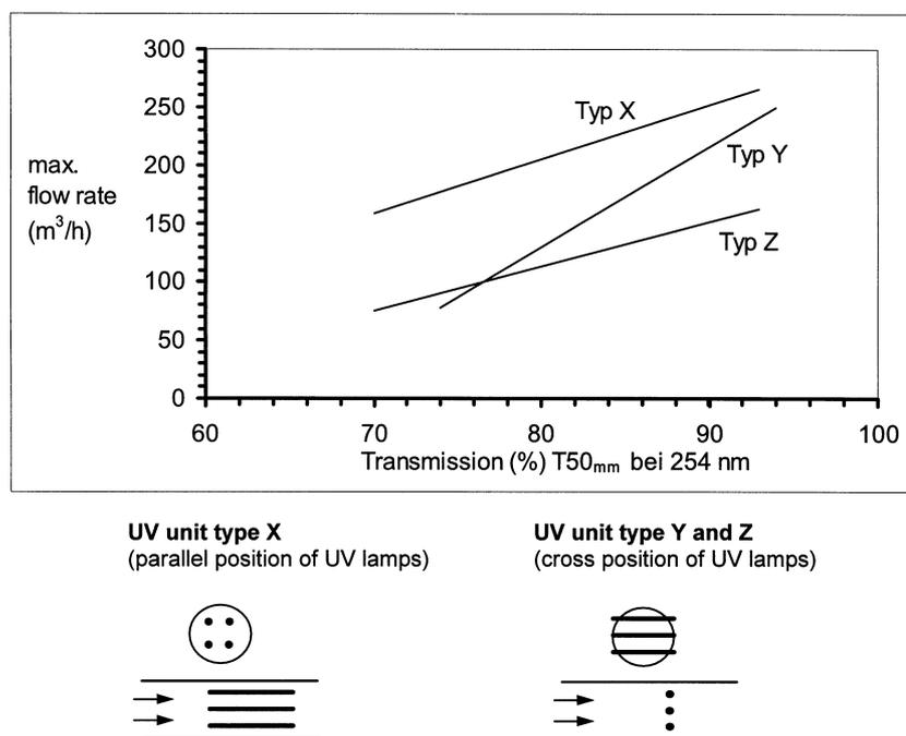
**Fig. 8** Influence of the reactor design and different types of UV lamps on the microbiological performance. In order to be directly comparable, the three sizing curves shown all represent a 400 J/m<sup>2</sup> UV dose.
