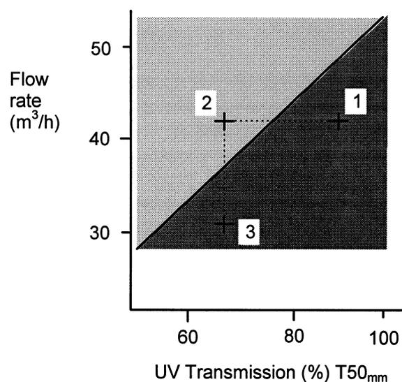
Fig. 1 Sizing curve of a UV unit.
