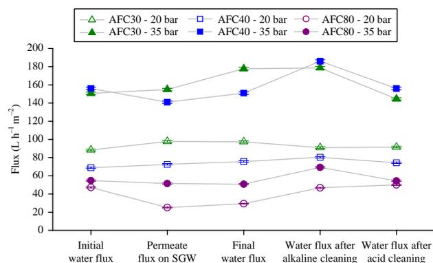
**Figure 2** | Flux evolution during filtration of SGW on AFC30, AFC40 and AFC80.
