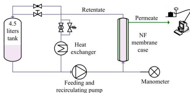
Figure 1 | Simple flow sheet of the NF pilot plant Microlab 40.
