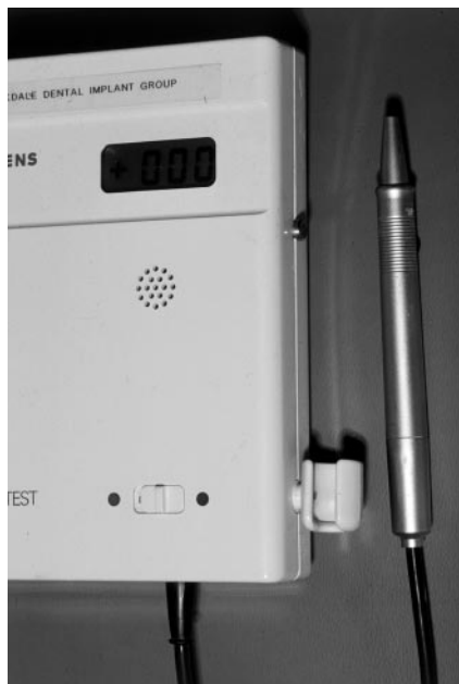
FIGURE 1. The Periotest apparatus consists of a control box and probe. The box contains a reporting window that indicates values. In addition, there is a corroborating verbal report that permits the operator to maintain eye contact with the site being tested.
