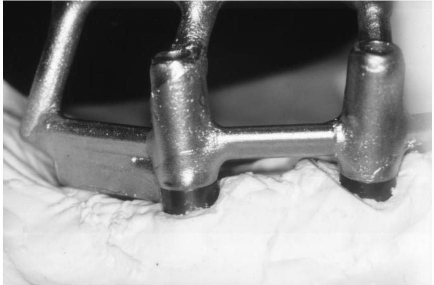
FIGURE 5. The fit of the casting after recovery. Williams Ivo-Clar IS 85 alloy was used.
