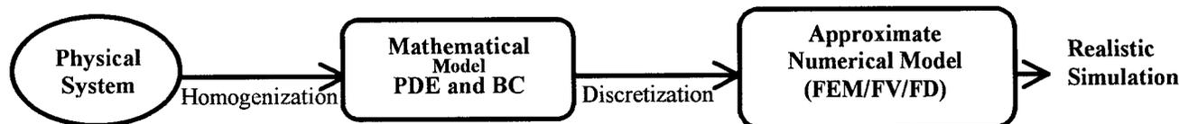
FIGURE 1. Overall computer simulation process. PDE indicates partial differential equations; BC, boundary conditions; FEM, finite element method; FV, finite volume; and FD, finite difference.
