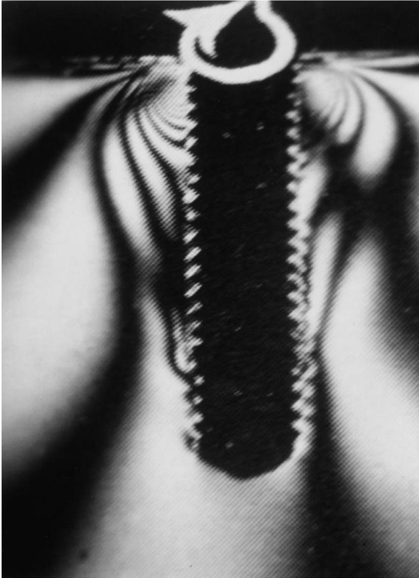
FIGURE 2. Photoelastic study of threaded implant in a bone simulant, which is torqued while in position. The stress contours are at the crestal region around the implant.
