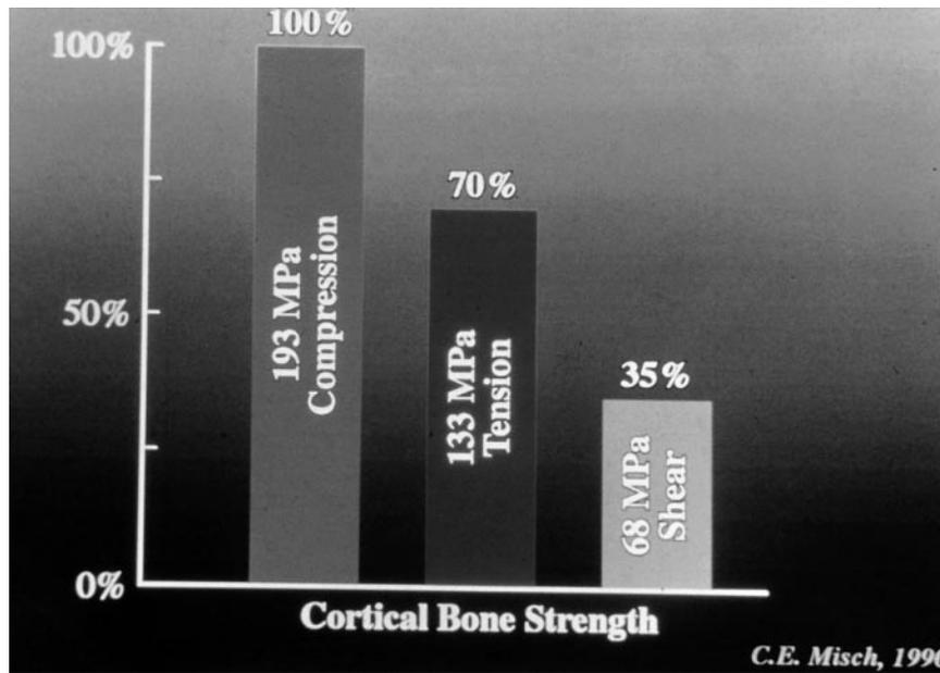
FIGURE 4. Bone is strongest in compression, 30% weaker in tension, and 65% weaker in shear. Torque forces apply shear to the implant-bone interface, especially at the crestal regions.
