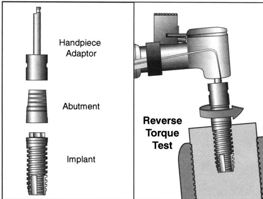
FIGURE 1. Schematic diagram of an *in vitro* reverse torque testing experiment.
