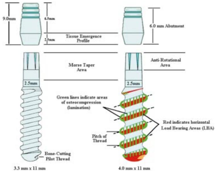
FIGURE 4. Note the different thread design. The larger pitch is designed as an aggressive thread having greater load-bearing areas for spongy bone, as noted in occlusal force to bone classification (*ie*, FB<sub>1</sub>; Table 2).
