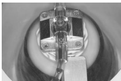
FIGURE 3. The centrifuge unit, at this point, is rotating at approximately 5600 rpm.
