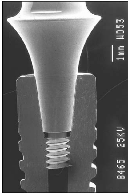
FIGURE 2. Precision-machined, internal-tapered abutment connection (Morse Taper) provides effective “anti-rotation” and eliminates micromovement during clinical function. The precise fit of this connection eliminates the microgap found in most 2-stage implant systems as well as food debris and bacteria that are often found in this microgap. Bacteria and micromovement are believed to be associated with crestal bone loss.
