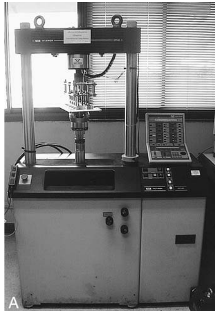
FIGURE 3. (A) Instron servohydraulic machine. (B) Ten specimens were simultaneously loaded. (C) Stylus on the indentation of the crown.
