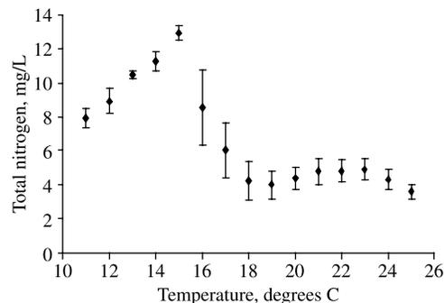
**Figure 1** Relationship between temperature and total nitrogen for Blue Plains' effluent (2004 data – 30 day rolling average)
