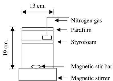
**Figure 4** Diagram of reactor
