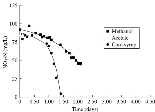
Figure 6 Temporal decrease of nitrate concentration with different substrates at  $19^\circ\text{C}$
