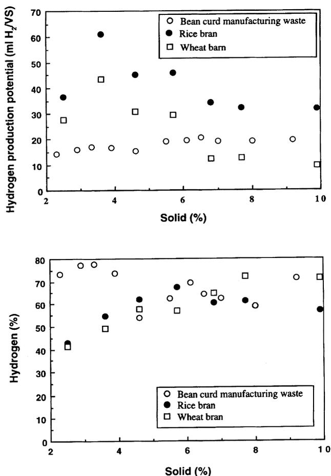
**Figure 1** The influence of solid concentration on hydrogen production potential and hydrogen percentage of the produced gas
