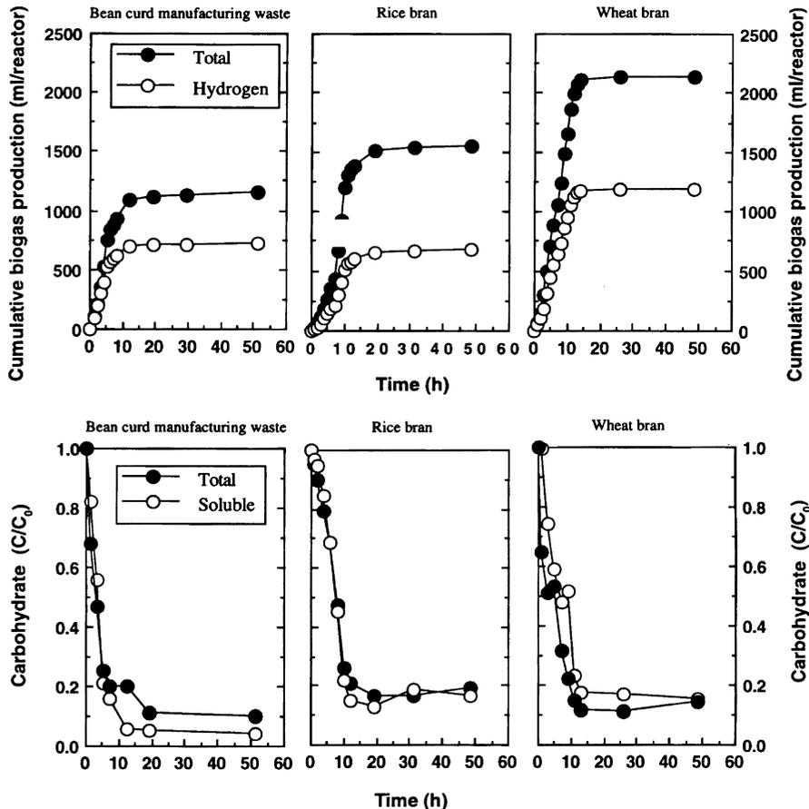
**Figure 2** Hydrogen production and decomposition of carbohydrate C, initial concentration of carbohydrate
