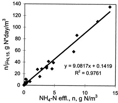
Figure 6 Determination of parameters in Monod model
