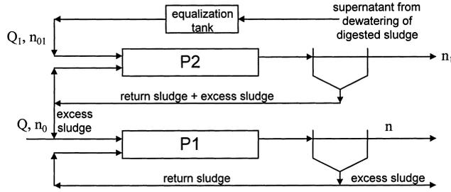
Figure 1 System with seeding of nitrification bacteria
