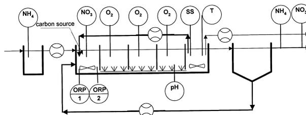
Figure 2 Layout of the pilot-scale activated sludge plant
