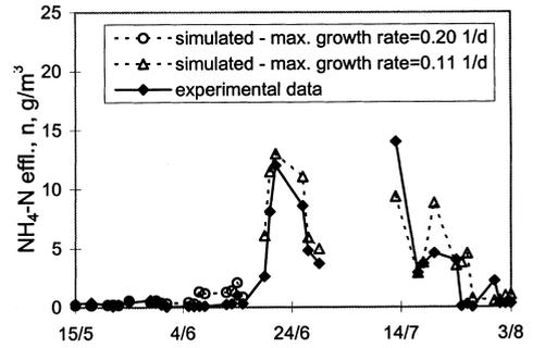
Figure 7 Verification of model with experimental data during seeding conditions:  $K_n=0.016 \text{ g N/m}^3$
