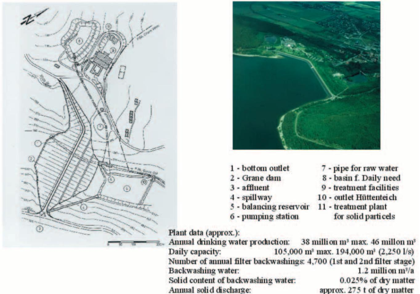
Figure 2 | Grane dam and connected plants.
