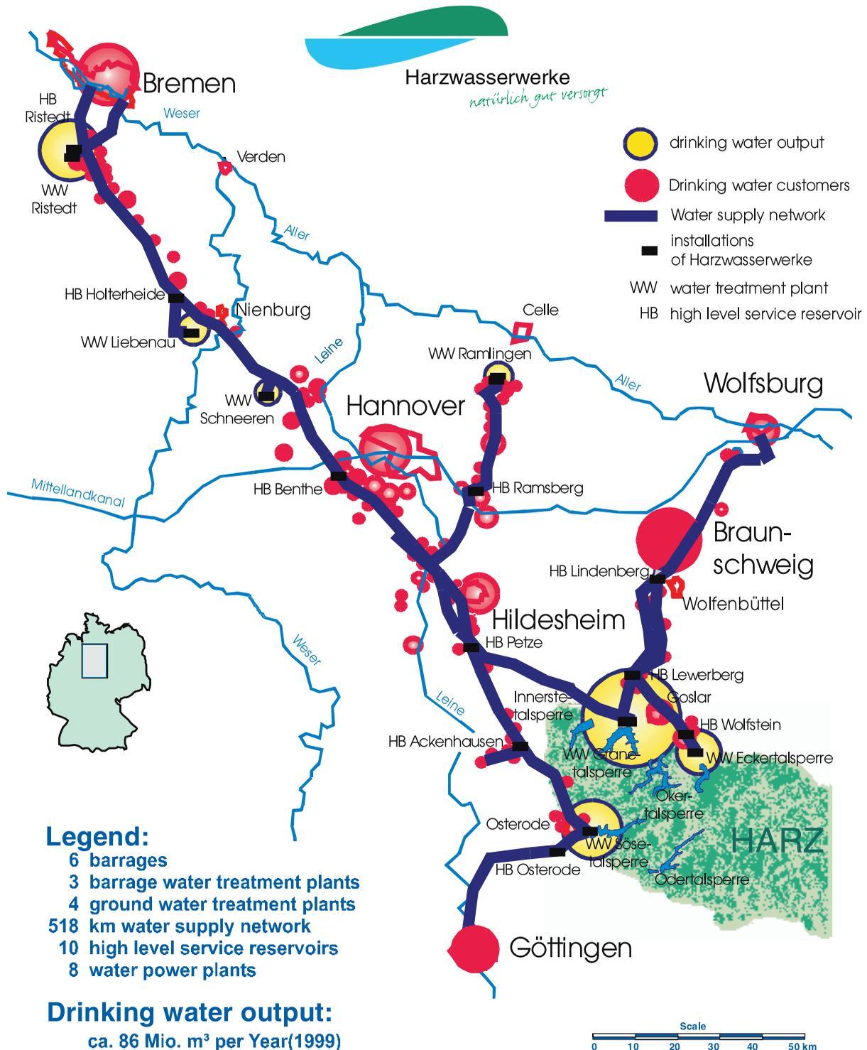
Figure 1 | Drinking water supply network of HARZWASSERWERKE GMBH.
