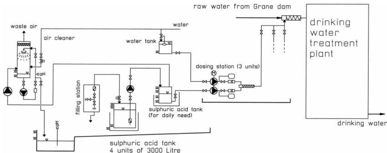
Figure 3 | Diagram of the sulphuric acid plant.
