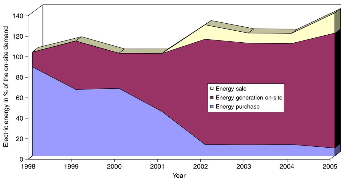
Figure 8 | Development of acquisition, generation and sale of electric energy.
