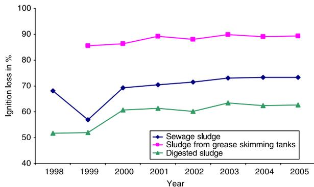
**Figure 5** | Ignition loss of sewage, grease interceptor and digested sludge.
