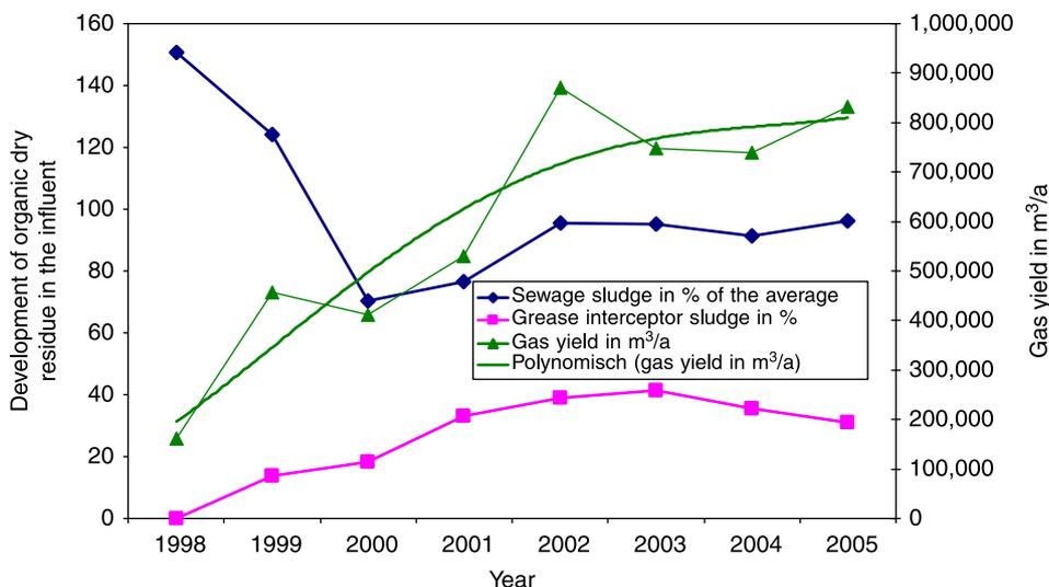
**Figure 6** | Relation between digestion of grease interceptor sludge and gas yield.
