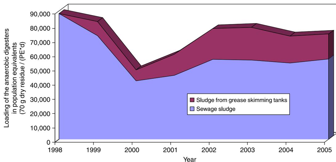
Figure 3 | Development of the loading of the digesters in terms of population equivalents.
