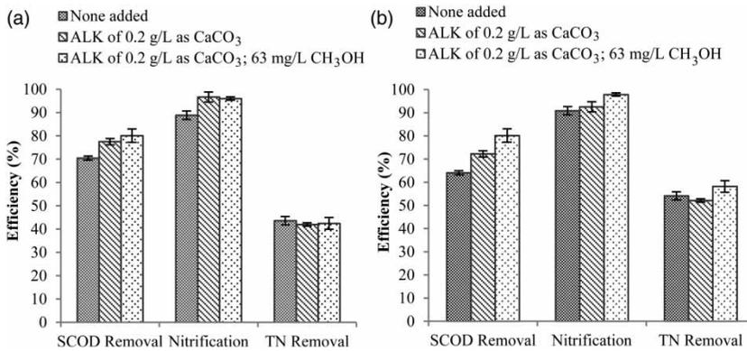
**Figure 4** | Effects of added ALK and electron donor (CH<sub>3</sub>OH) at different PR of (a) 19% and (b) 31% on C and N removals from MW. (a): PR, 19%; HRT, 6 h; SCOD<sub>0</sub>, 50–83 mg/L; NH<sub>3</sub>-N<sub>0</sub>, 16–26 mg/L; continuous aeration; pH, 6.3–8.0; DO, 7.6–8.2 mg/L, (b): PR, 31%; HRT, 6 h; SCOD<sub>0</sub>, 49–100 mg/L; NH<sub>3</sub>-N<sub>0</sub>, 20–30 mg/L; continuous aeration; pH, 6.5–7.8; DO, 6.6–8.1 mg/L.
