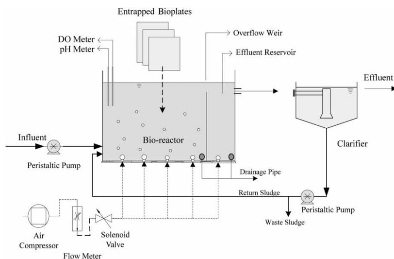
**Figure 2** | Schematic diagram of (a) entrapped biomass system and (b) a clarifier to couple with conventional AS system.
