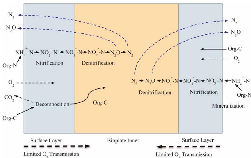
Figure 1 | C and N removal mechanisms with entrapped biological process with oxic/anoxic/anaerobic transitions.
