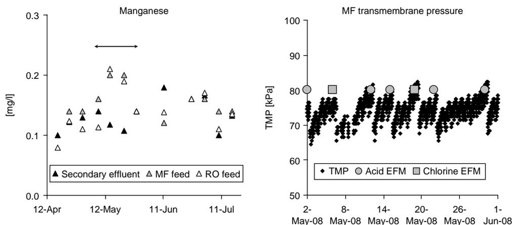
Figure 1 | Manganese residual in MF and RO feed waters (left) versus MF TMP (right).
