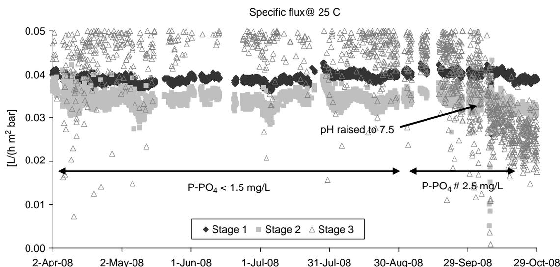
Figure 2 | RO specific flux during a scaling event.
