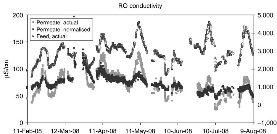
**Figure 4** | Conductivity trends over the trial period: RO feed, RO permeate (actual, and normalised).
