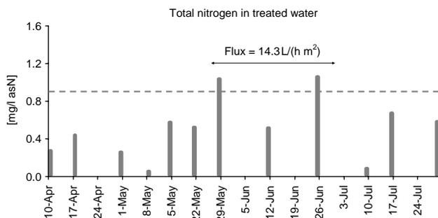
**Figure 3** | Total nitrogen concentration in RO permeate, at 18.0 L/(h m<sup>2</sup>), and 14.3 L/(h m<sup>2</sup>).
