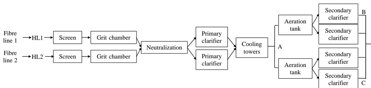
**Figure 2** | Flow diagram of high organic load effluent treatment at the mill, indicating locations of effluent sampling points. (A-primary effluent; B-treated effluent, system 1; C-treated effluent, system 2).
