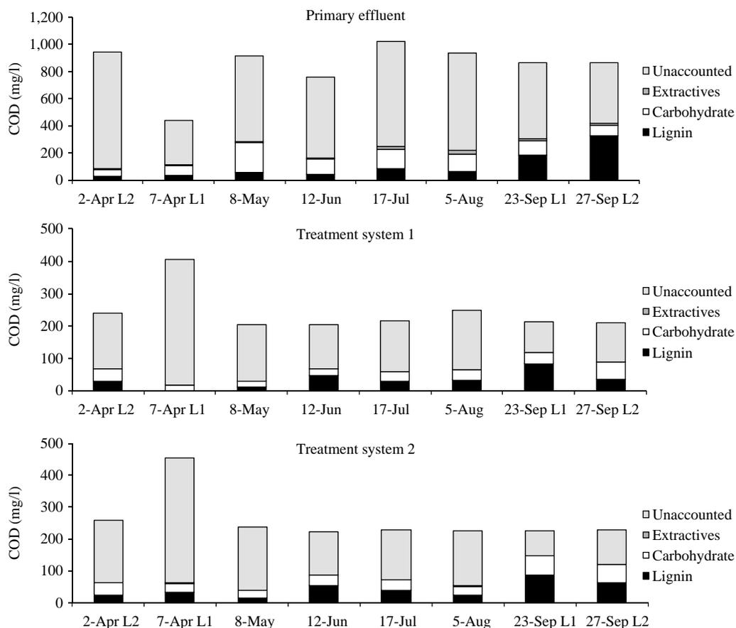
**Figure 3** | Chemical oxygen demand (COD) components in primary and biologically treated bleached kraft pulp effluent in activated sludge treatment systems 1 and 2 during normal mill operation and mill maintenance shutdowns. (L1 or L2 after the sample date indicates which fibre line was under maintenance shutdown during sampling).
