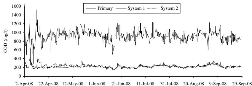
**Figure 1** | COD profiles of primary (upper trace) and biologically treated effluent during a six-month monitoring period, including two maintenance shutdowns (in April and September). (Systems 1 and 2 refer to treated effluents from the parallel treatment systems).
