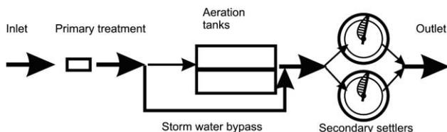
Figure 1 | Flow scheme for the storm water bypass process.
