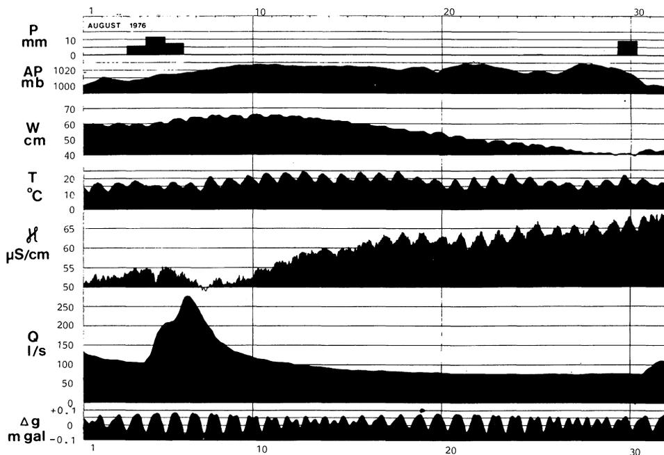
Fig. 2. Variation of a number of parameters at station A (Fig. 1) in August 1976. P) precipitation AP) atmospheric pressure W) groundwater stage T) water temperature K) electrical conductivity of water at 20°C Q) water discharge  $\Delta$  g) gravity variation.
