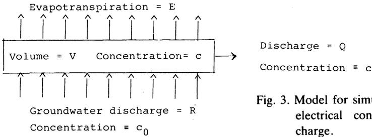
Fig. 3. Model for simulating variations in electrical conductivity and discharge.
