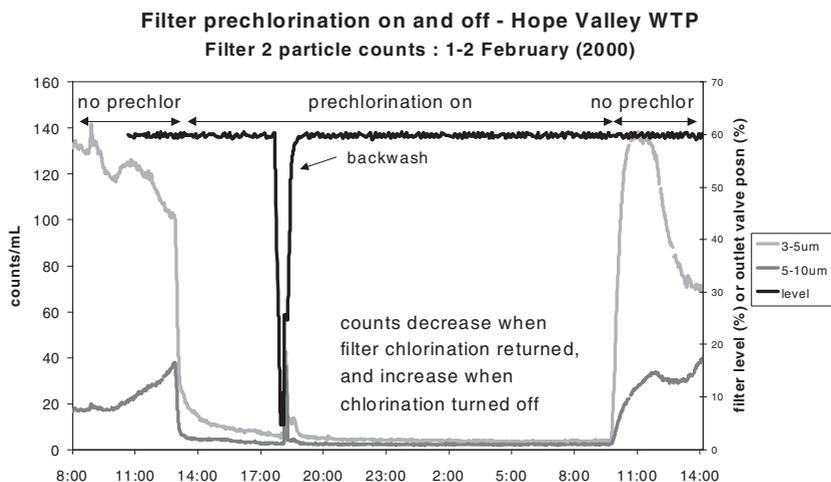
**Figure 2** Filter pre-chlorination and filtered water particle count
