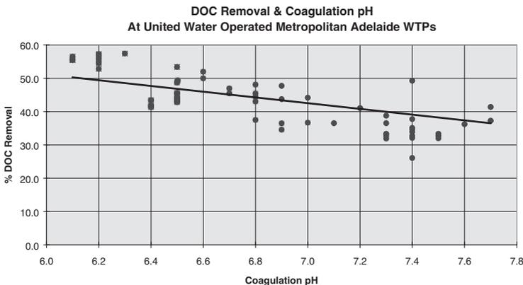
**Figure 1** Coagulation pH and DOC removal
