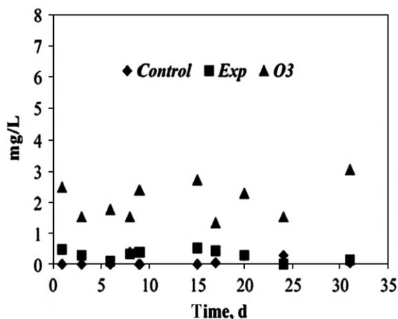
**Figure 5** Soluble ammonia nitrogen in the activated sludge at the end of the react phase and after ozone treatment in SBRs
