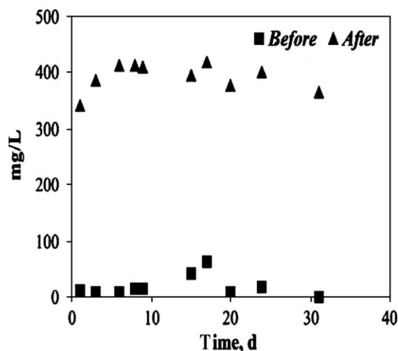
**Figure 4** Soluble COD concentration in the activated sludge before and after ozone treatment
