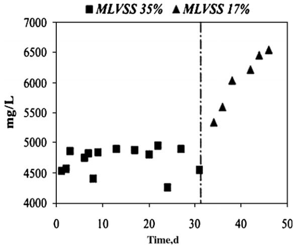
**Figure 2** MLVSS concentration in Exp SBR for 0.05 gO<sub>3</sub>/gSS (35%) and 0.025 gO<sub>3</sub>/gSS (17%)
