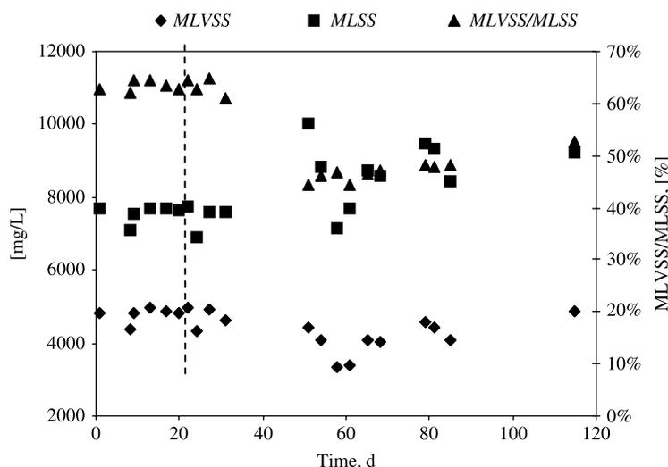
Figure 1 MLSS and MLVSS concentration and MLVSS/MLSS ratio in Exp SBR
