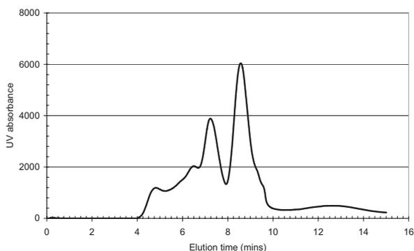
**Figure 2** Typical molecular size profile for grey water
