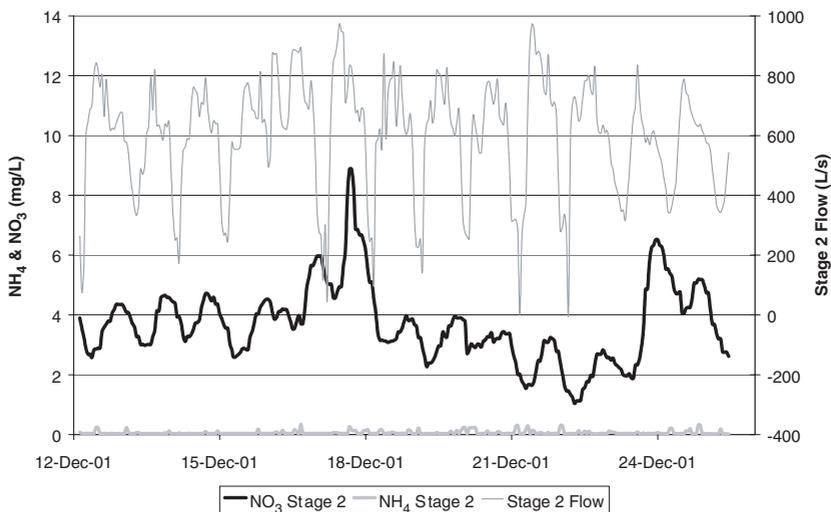
**Figure 5** Stage 2 on-line nutrient analyser trends showing weekly nitrate variation
