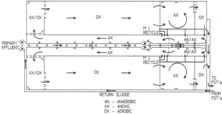
**Figure 2** Five stage Bardenpho bioreactor layout for Luggage Pt WWTP N removal upgrade
