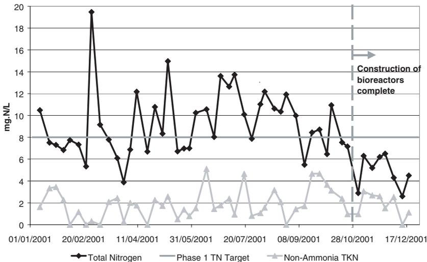
**Figure 3** Effluent nitrogen for Luggage Pt WWTP during construction and commissioning
