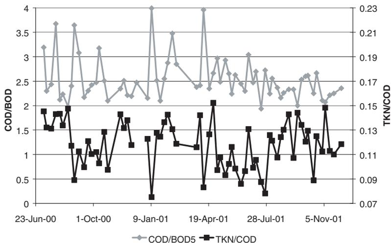
**Figure 1** Primary settled effluent COD/BOD<sub>5</sub> and TKN/COD ratios for Luggage Pt WWTP
