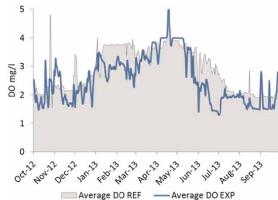
**Figure 5** | Daily DO concentration in reference lines (REF, constant DO control) and experimental lines (EXP, ammonium feedback control) at Henriksdal WWTP during the 1 year experiment.
