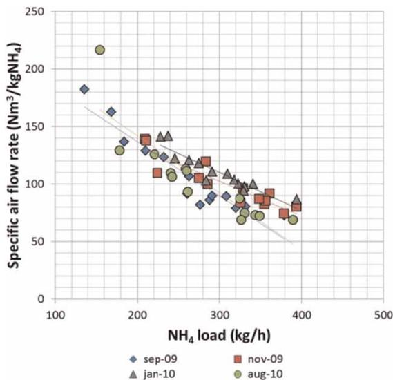
**Figure 6** | Specific air flow rate as a function of ammonium load for 2 cold and 2 warm months. Data from Henriksdal WWTP.
