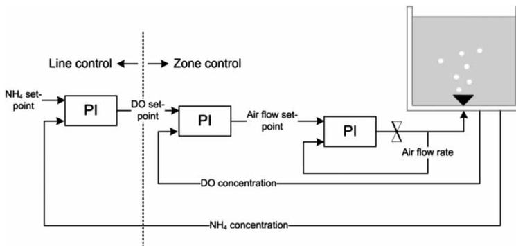
**Figure 2** | Cascade control of ammonium. One ammonium controller determines the DO set-point of several aerated zones.
