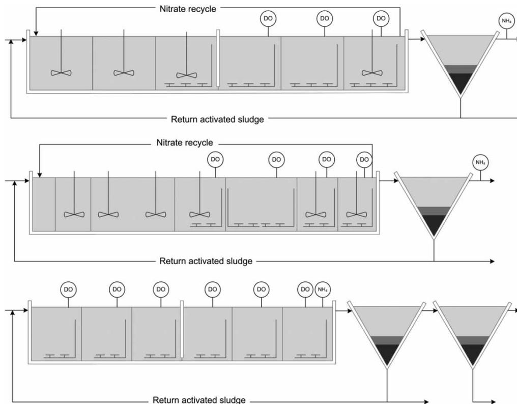
Figure 1 | The activated sludge processes and instrumentation in the experimental lines. Top: Henriksdal WWTP, middle: Käppala WWTP and bottom: Himmerfjärden WWTP.
