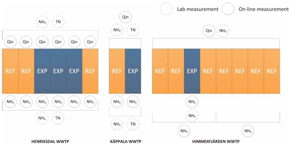
**Figure 3** | Summary of experimental set-up and instrumentation for Henriksdal WWTP (left), Käppala WWTP (middle) and Himmerfjärden WWTP (right). REF = reference line, EXP = experimental line, Qin = inflow rate, TN = total nitrogen, NH<sub>4</sub> = ammonium.
