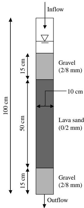
Figure 1 | Scheme of the sand filter column.
