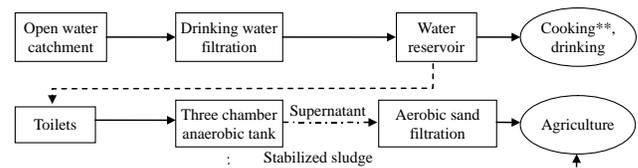
Figure 2 | Scheme of the proposed drinking water and wastewater treatment system in Glompong. \*\*Boiling the water is usual in Indonesia as disinfection treatment.
