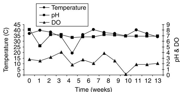
Figure 1 | Graphical representation of pH, temperature and dissolved oxygen (DO) in the SMBR.
