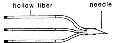
**Figure 2**—Filtrate collector as used in this study
