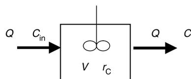
Figure 1 | System of a completely stirred reactor.
