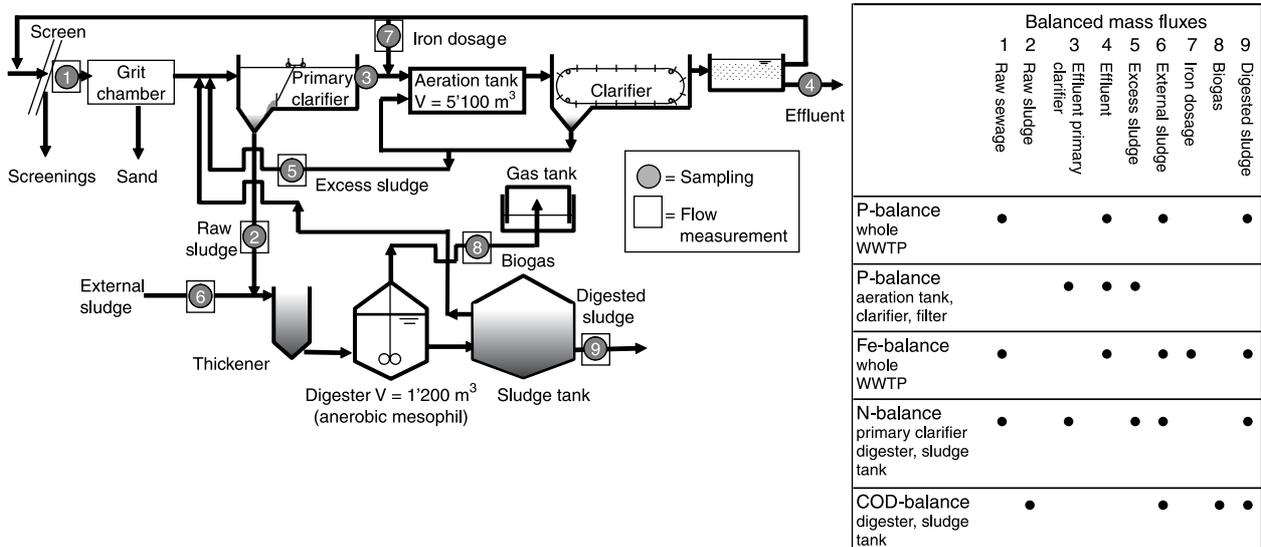
Figure 4 | WWTP Ergolz 1 with analyzed mass balances.
