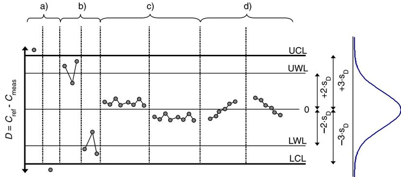
Figure 6 | Shewhart control charts with less stringent out-of-control criteria for the warning phase and normally used criteria (Montgomery 1996) for the alarm phase.
