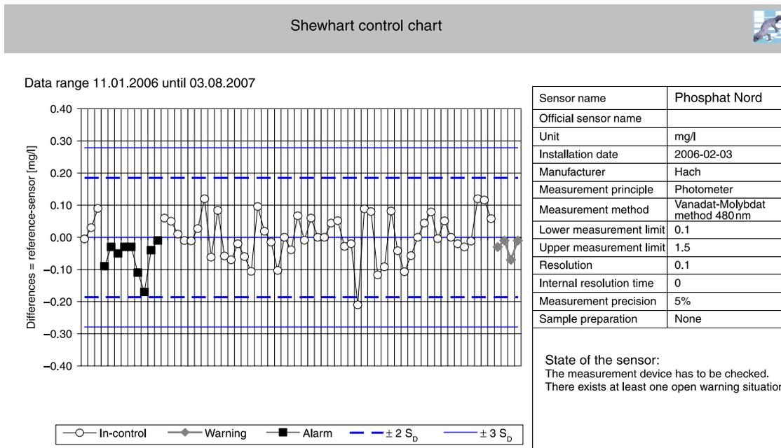
Figure 7 | Example of a Shewhart control-chart for  $\text{PO}_4\text{--P}$ , effluent filter north, WWTP Zürich-Werdhölzli, out-of-control situations are marked with bold squares.
