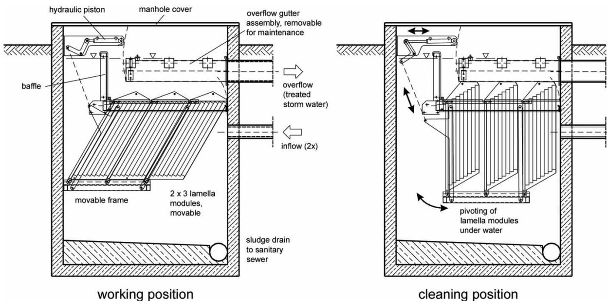
**Figure 4** | For cleaning, the lamella modules are pivoting under water by a hydraulic drive. The sludge slides down and is drained to a sanitary sewer.
