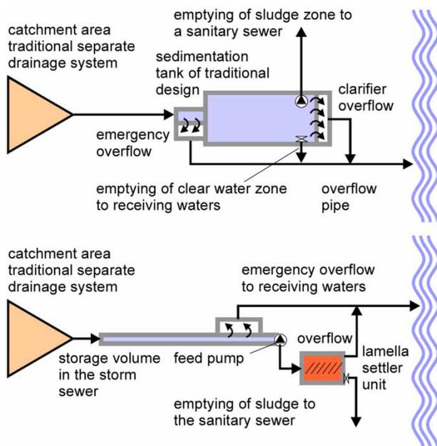
**Figure 2** | Top: traditional sedimentation tank which is emptied after each storm event. Bottom: alternative concept where the storm sewer is used as a storage volume, plus a lamella settler as treatment device.
