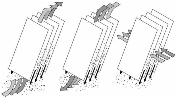
**Figure 1** | Lamella settlers of counter-flow, parallel flow and cross-flow type.
