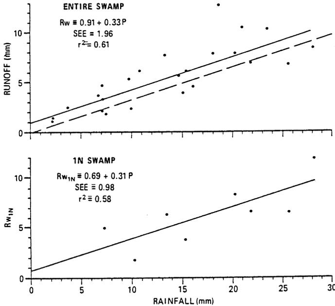
Fig. 5. Basin swamp, 1987 and 1988, and 1N swamp, 1987, stormflow runoff versus storm precipitation.  $R$ ,  $P$ ,  $SEE$  and  $r^2$  signify, respectively, runoff and precipitation (mm storm<sup>-1</sup>), standard error of the estimate (mm storm<sup>-1</sup>) of  $R$  using the regression equation, and the coefficient of explanation.
