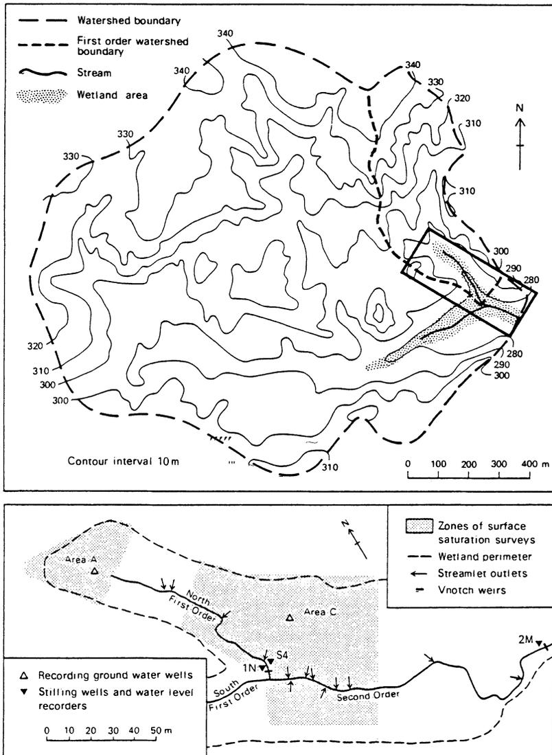
Fig. 1. Upper: The topography of the study basin and the location of the treed spring-fed swamp in the valley bottom. The enclosed rectangle indicates the location of the enlarged are display below. Lower: Location of the water level recording sites and the area of the surface saturation survey.
