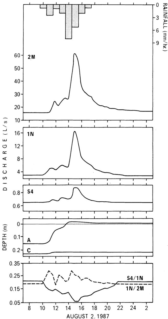
Fig. 7. The storm hydrographs for the basin, 1N, and 2M outlets, water table elevation relative to the ground surface for Areas A and C, and hourly rainfall distribution for August 2, 1987.
