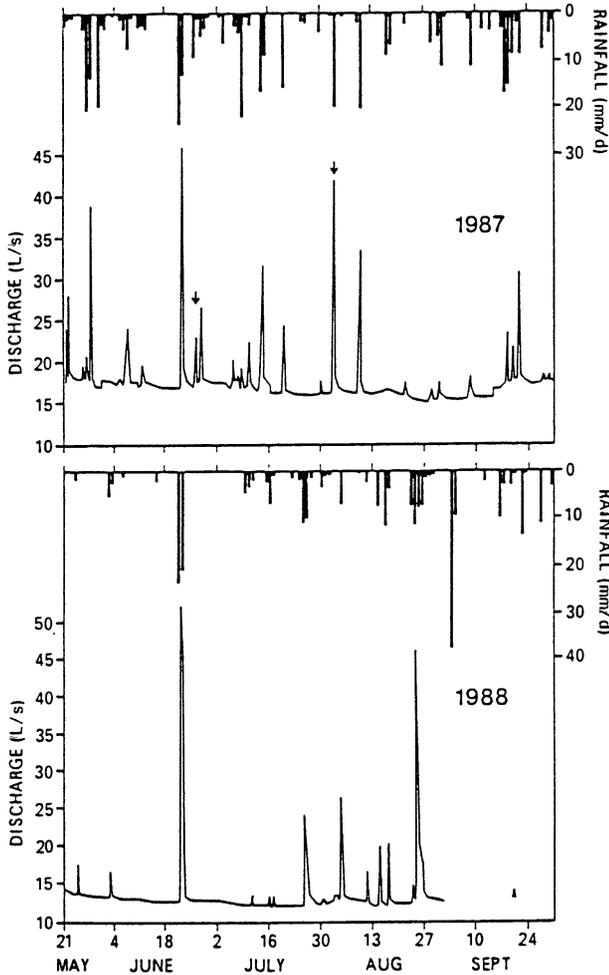
Fig. 4. Summer outlet (2M) streamflow hydrograph and rainfall for 1987 (upper box) and 1988 (lower box). The arrows on the 1987 hydrograph indicate the storms shown in detail in Figs. 6 and 7.
