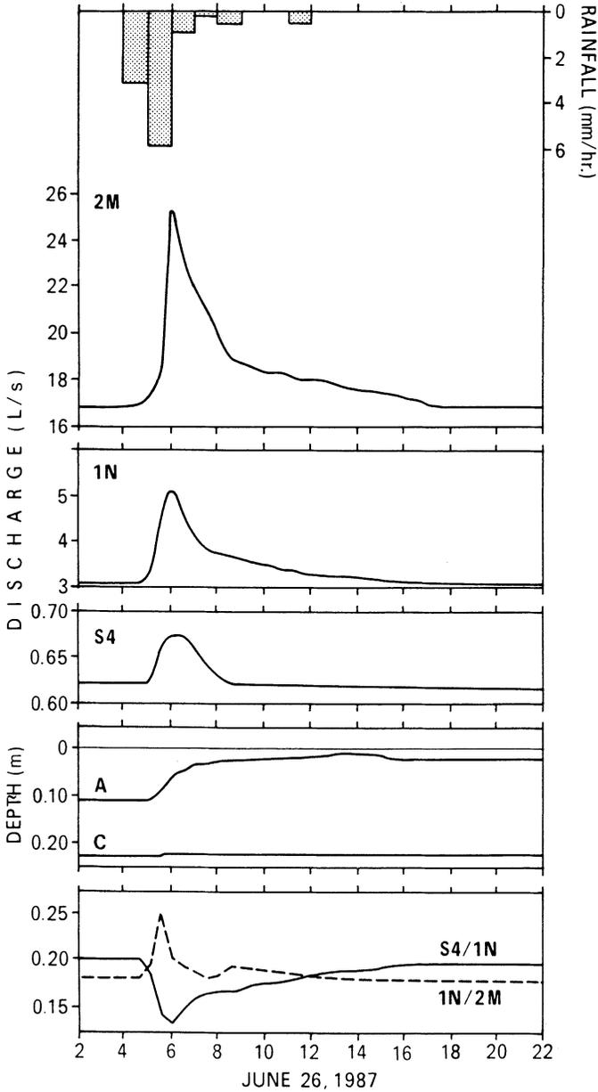
Fig. 6. The storm hydrographs for the basin, 1N, and 2M outlets, water table elevation relative to the ground surface for Areas A and C, and hourly rainfall distribution for June 26, 1987.
