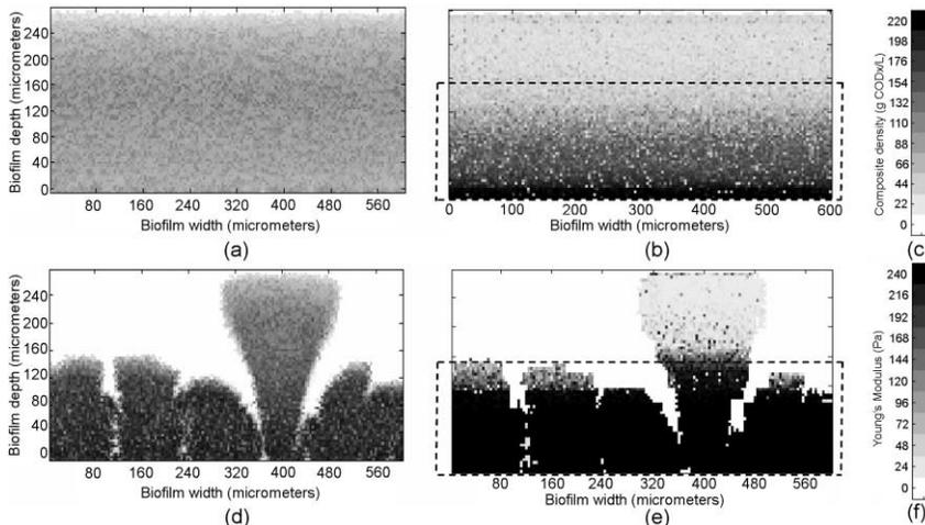
**Figure 1** Composite density plots: (a) for biofilm I and (d) for biofilm II, composite Young's modulus ( $E_{comp}$ ): (b) for biofilm I and (e) for biofilm II. Corresponding shading scales: (c) for composite density and (f) for Young's modulus. Dashed line encloses sections input in ABAQUS
