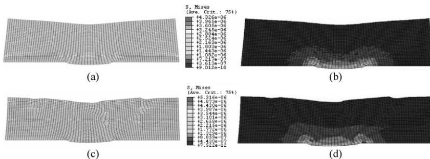
**Figure 3** (a) Deformed biofilm I and (c) biofilm II under tensile load conditions, showing FE mesh. (b) Graphical output of von Mises stresses distribution of biofilm I and (d) biofilm II
