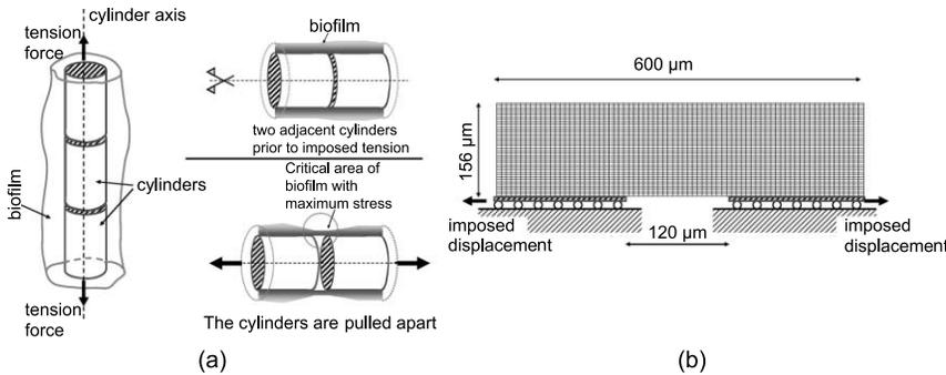
**Figure 2** (a) Schematic representation of the loading conditions, motivated by the experiments of *Ohashi et al. (1999)*. (b) FE mesh and boundary conditions employed in the present analysis
