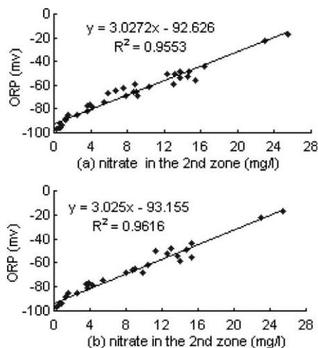
**Figure 2** The correlation between ORP and nitrate concentration in the second zone of different (a) nitrate recirculation flow and (b) external carbon dosage
