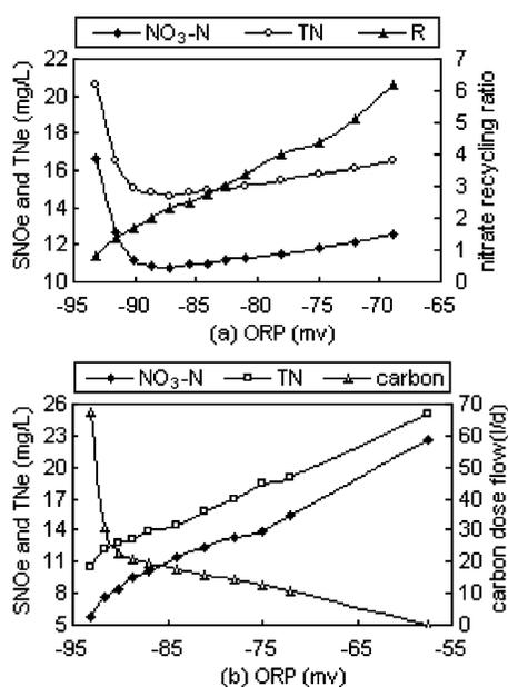
**Figure 3** The effect of (a) nitrate recirculation flow and (b) external carbon dosage on the effluent nitrate and TN, and the ORP value at the end of the anoxic zone
