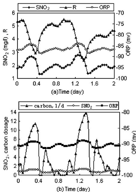
**Figure 5** The results of fuzzy controllers, (a) nitrate in the second zone, ORP and nitrate recirculation flow ratio; (b) nitrate in the second zone, ORP and external carbon dosage
