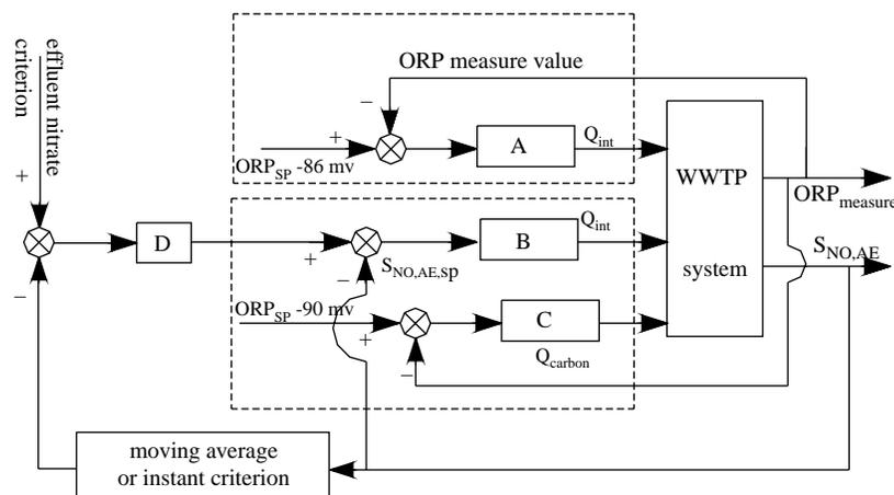
**Figure 6** The combined control structure of nitrate recirculation and external carbon addition
