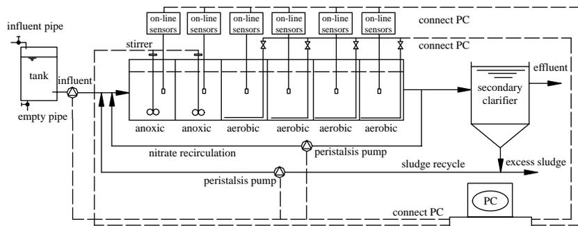
Figure 1 Schematic diagram of a predenitrification process
