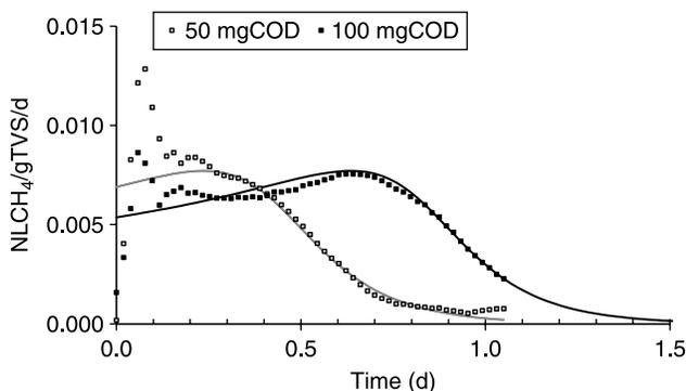
**Figure 4** | Experimental SMA on acetate fitted by a Haldane kinetics model.
