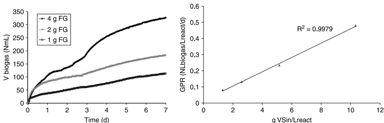
**Figure 6** | Net biogas production in test with increasing doses of grass (left), Average gas production rate (GPR) in test with increasing doses of grass (right).
