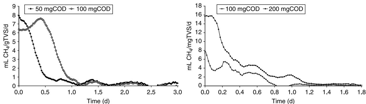
**Figure 3** | Net SMA trends in acetate (on the left) and glucose (on the right) methanization tests.
