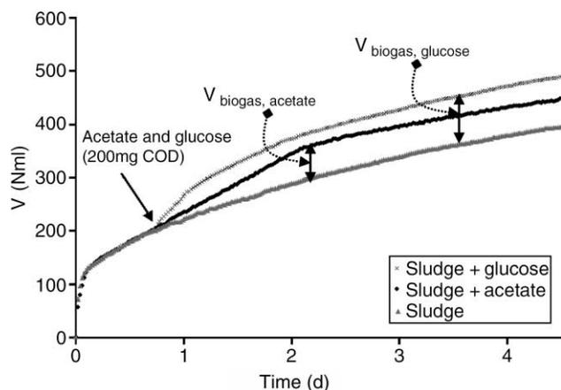
**Figure 2** | Biogas production measured after acetate and glucose addition in a lab-scale test with a low F/M ratio.
