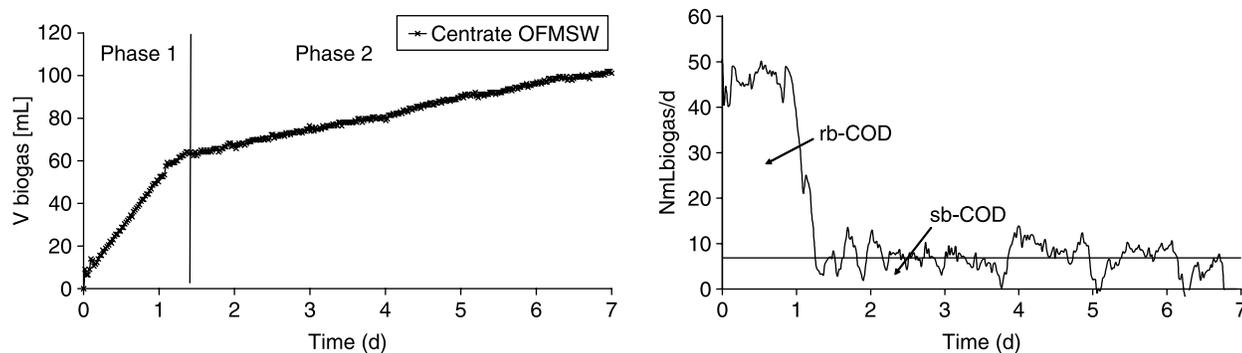
**Figure 7** | left Net biogas production in test with 2 ml of C-KW (left), net biogas production rate in test with C-KW (right).
