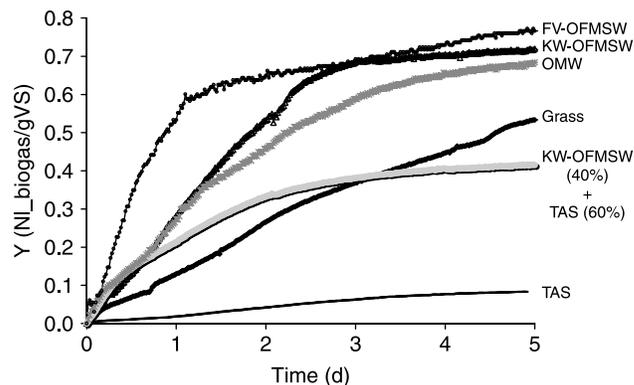
**Figure 5** | Example of specific biogas production registered during batch tests on various organic substrates.
