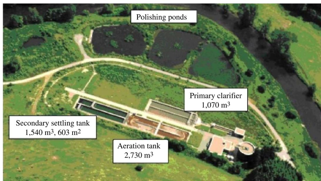
**Figure 1** | Plant layout of the Finntrop WWTP before upgrading.
