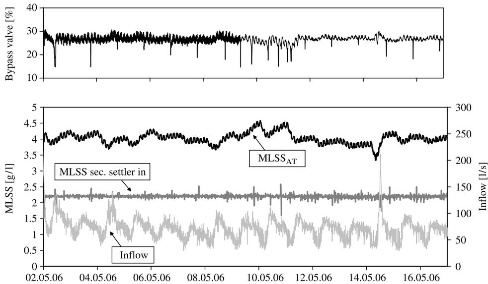
**Figure 5** | Suspended solids concentration in the activated sludge tank and in the influent of the secondary settling tank under dry weather conditions.
