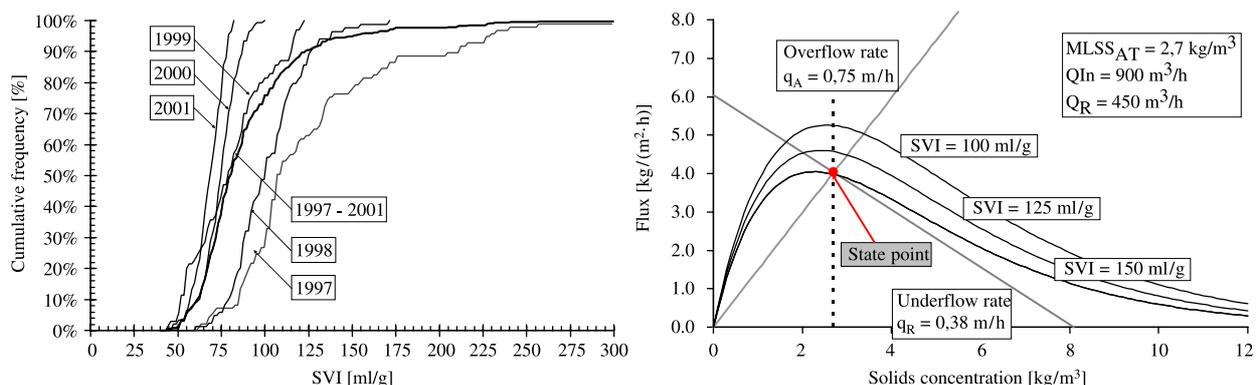
**Figure 2** | Frequency distribution of sludge volume index and operating chart for the secondary settling tank.
