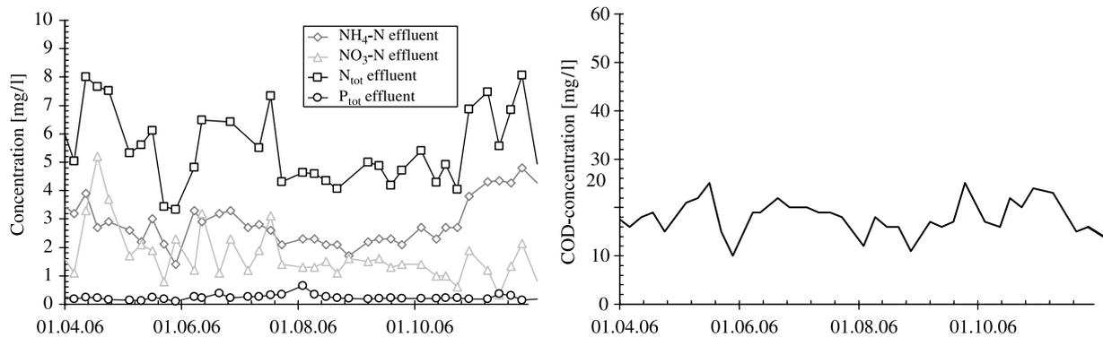
Figure 7 | Nutrient and COD concentrations in the effluent after optimisation of the lamella operation.
