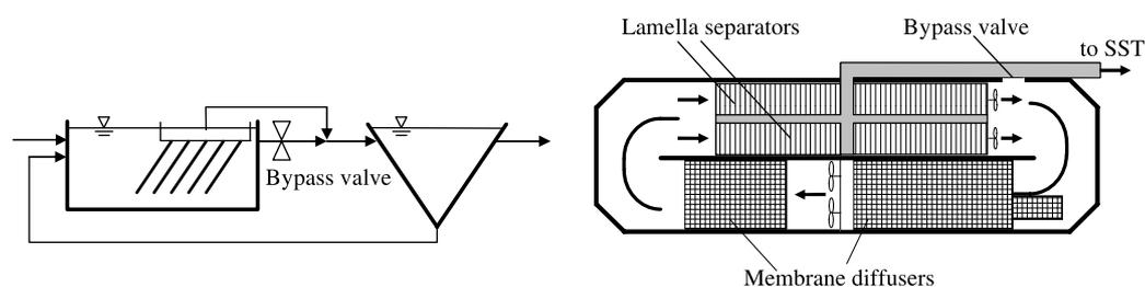
**Figure 3** | Schematic diagram of the bypass valve (left) and schematic layout of the activated sludge tank equipped with four lamella separators and membrane diffusers (right).
