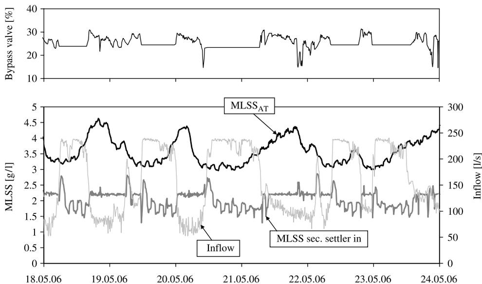
**Figure 6** | Suspended solids concentration in the activated sludge tank and in the influent of the secondary clarifier during wet weather conditions—horizontal lines in the upper graph show the fixed opening of the bypass valve at flow rates above 150 l/s.
