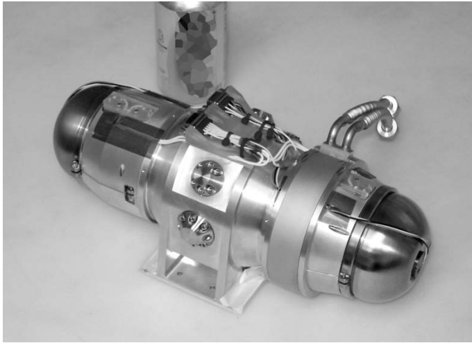
FIGURE 2: Lockheed Martin M5 Midi compressor. This TRL 6 compressor has a mass of 6 kg and an input power capability of 600 W electrical power. During this testing, the compressor demonstrated 75% efficiency with 600 W electrical input power, and 85% efficiency with 200 W electrical input power. A 12-ounce soda can is shown in the background for size comparison.
