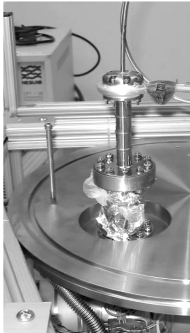
FIGURE 1: Prototype high capacity pulse tube coldhead. The regenerator is below the bolted copper cold flange, obscured by MLI. The pulse tube is above the cold flange. The aftercooler is in a copper flange below the regenerator, which forms part of the vacuum seal.
