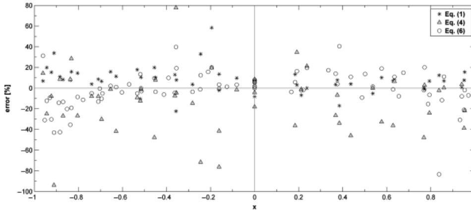
**Figure 7** | Percentage error in estimating the mean velocity along the 80 sampled verticals assuming velocity points sampled only in the upper portion of flow area (high flow). Distance  $x'$  represents the dimensionless horizontal distance of each vertical from that in which  $u_{\max}$  was observed ( $x=0$ ).
