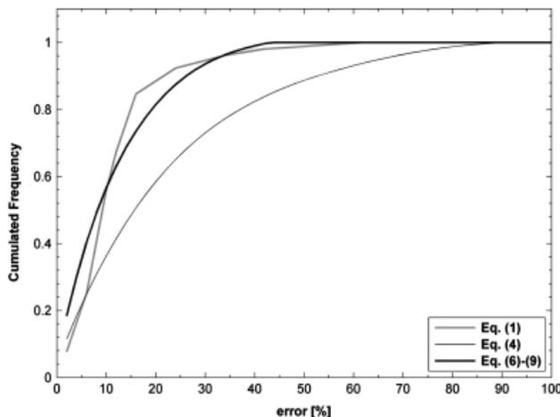
**Figure 8** | Cumulated frequency of the percentage error, in magnitude, in estimating the mean velocity along the 80 investigated verticals, considering the sampling of velocity points in the upper portion of flow area (high flow). Errors referring to Equations (6) and (9) are assessed considering the sampling of  $u_{\max}$  only.
