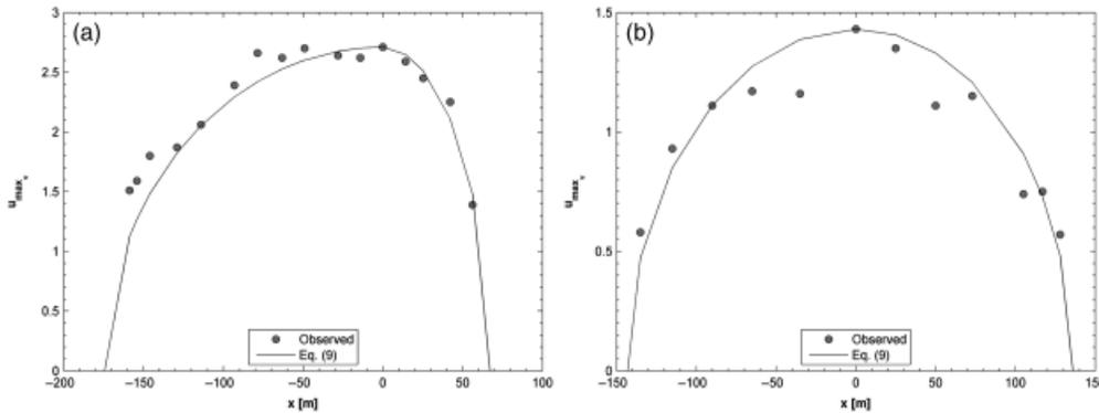
**Figure 4** | Elliptical distribution, Equation (9), of the maximum velocities,  $u_{max}$ , along verticals plotted against the observed ones for the flood event of (a) 16 October 1987 and (b) 24 February 1987.
