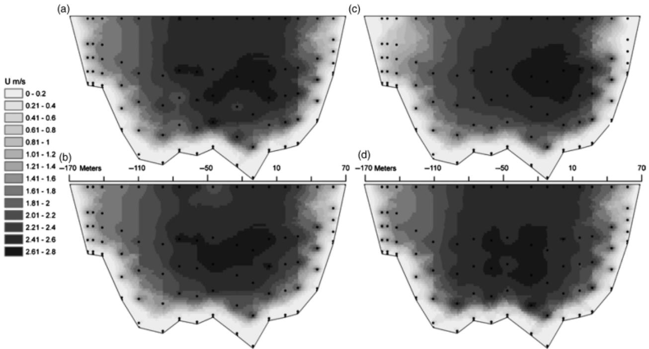
**Figure 5** | Flood Event on 27 February 1987. Spatial distribution of flow velocity obtained by (a) sampled velocity points, (b) Equation (6) using the velocity points sampled in the upper portion of the flow area, (c) Equation (6) coupled to Equation (9), and (d) Equation (1). Sampled velocity points are also shown.
