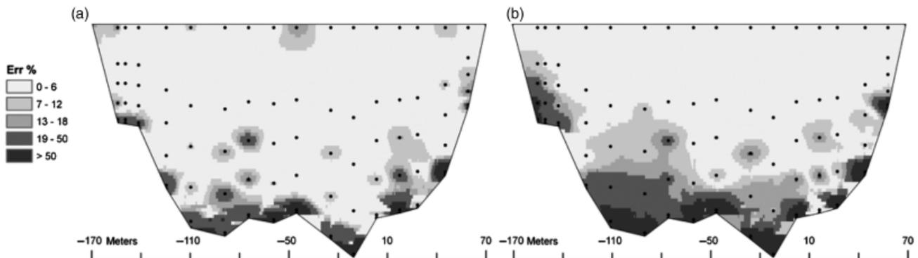
**Figure 6** | Flood Event on 27 February 1987. Percentage errors in estimating the flow velocity spatial distribution by using (a) Equation (6) with maximum velocity sampled along each vertical and (b) Equation (1).
