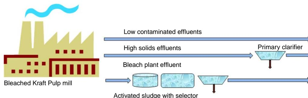
**Figure 1** | Mill case, showing a bleached Kraft Pulp mill with a production of 400,000 ADt/year.
