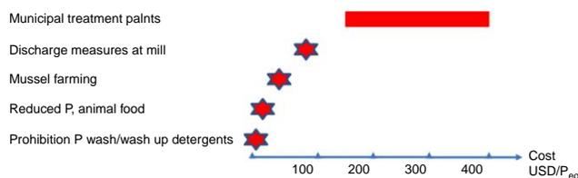
**Figure 3** | Costs for  $P_{eq}$  reduction by different methods.
