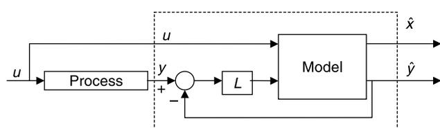
Figure 1 | Observer system overview (part within dashed area is called the observer).
