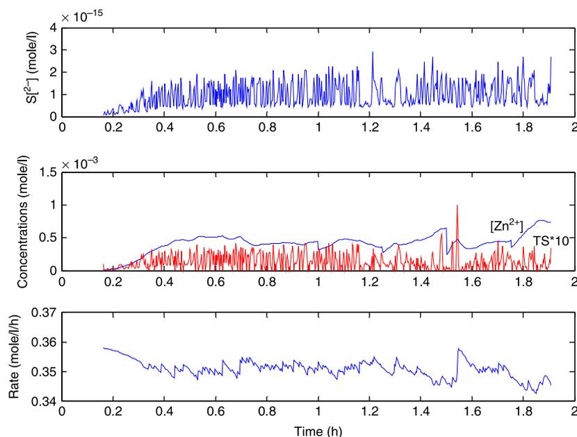
**Figure 3** | Observer performance using experimental data of  $[S^{2-}]$  and  $[Zn^{2+}]$ .
