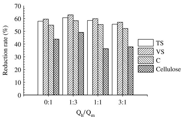
Figure 6 | Reduction rate of VS, TS, carbon and cellulose.
