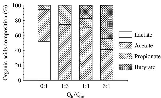
Figure 5 | Speciation of organic acids in the hydrolytic effluents.
