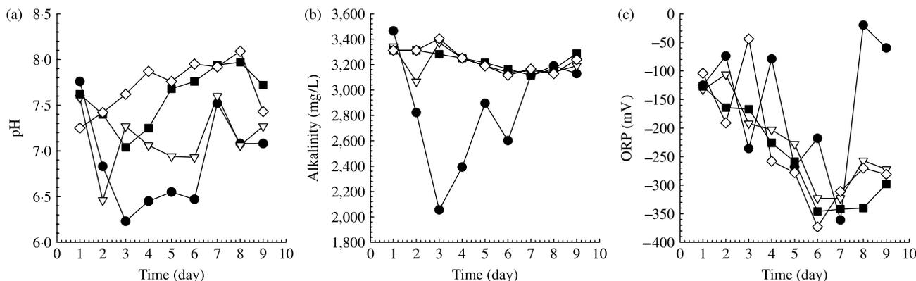
Figure 2 | Temporal evolution of pH, alkalinity and ORP. (a) pH; (b) Alkalinity; (c) ORP. ●  $Q_r$   $0.1 \text{ m}^3/(\text{m}^3 \cdot \text{d})$ ; ▽  $Q_r$   $0.5 \text{ m}^3/(\text{m}^3 \cdot \text{d})$ ; ■  $Q_r$   $1.0 \text{ m}^3/(\text{m}^3 \cdot \text{d})$ ; ◇  $Q_r$   $2.0 \text{ m}^3/(\text{m}^3 \cdot \text{d})$ .
