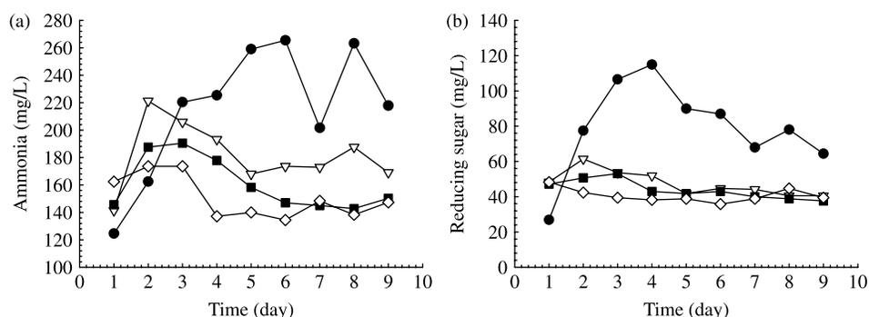
**Figure 3** | Temporal evolution of ammonia and reducing sugar. (a) Ammonia; (b) Reducing sugar. ●  $Q_r$  0.1  $\text{m}^3/(\text{m}^3\cdot\text{d})$ ; ▽  $Q_r$  0.5  $\text{m}^3/(\text{m}^3\cdot\text{d})$ ; ■  $Q_r$  1.0  $\text{m}^3/(\text{m}^3\cdot\text{d})$ ; ◇  $Q_r$  2.0  $\text{m}^3/(\text{m}^3\cdot\text{d})$ .
