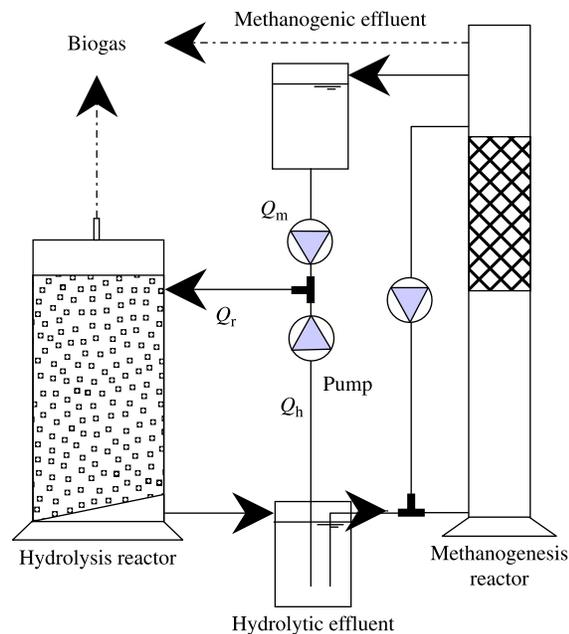
**Figure 1** | Scheme of the reactors for two-phase anaerobic digestion.
