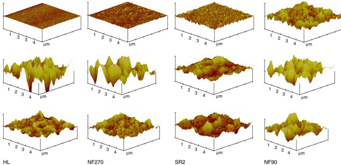
**Figure 4** | AFM images (45° view) of virgin (top) and fouled membranes fed with GRW (middle) and FRW (bottom) (scan area 5 μm × 5 μm).
