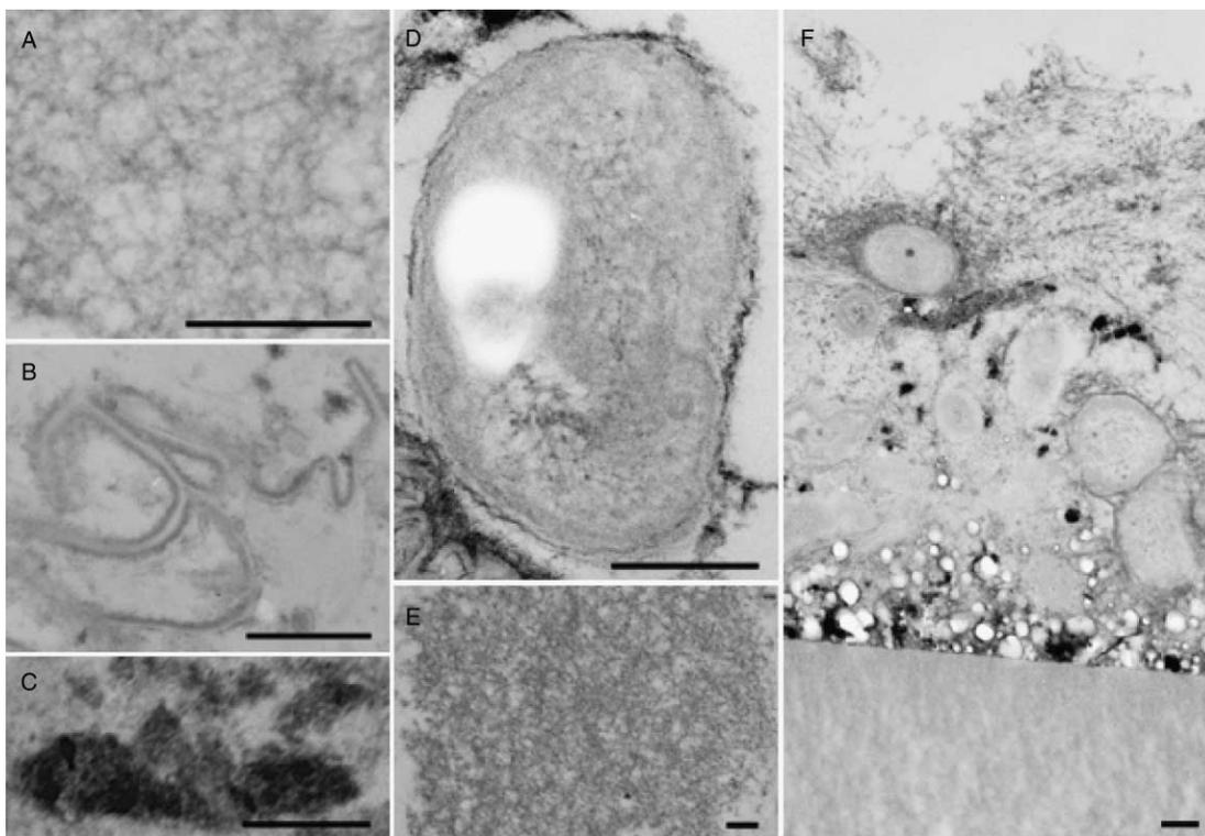
**Figure 8** | Photographs of fibrils (A), cellular debris (B), inorganic foulants (C), bacterium (D), humics (E) and typical fouling layer on the active layer of all membranes (scale bar 200 nm).
