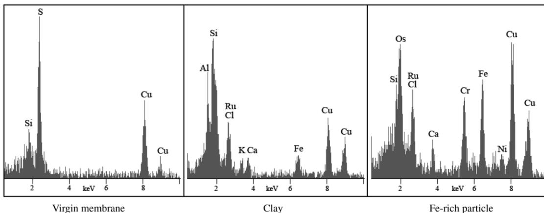
**Figure 10** | EDS spectra of virgin NF90 membrane and particles located on the active layer after filtration of GRW (Y scale 200).
