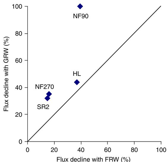
**Figure 2** | Comparison of flux decline at 10 gC/m<sup>2</sup> loading for GRW and FRW.
