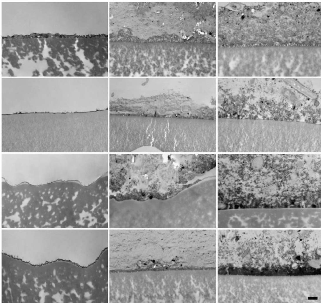
**Figure 9** | TEM images (Magnification 10K $\times$ , scale bar 500 nm) of virgin membranes (first column), fouled membranes fed with GRW (second column) and fouled membranes fed with FRW (third column) (NF90, HL, NF270 and SR2 from top to bottom).
