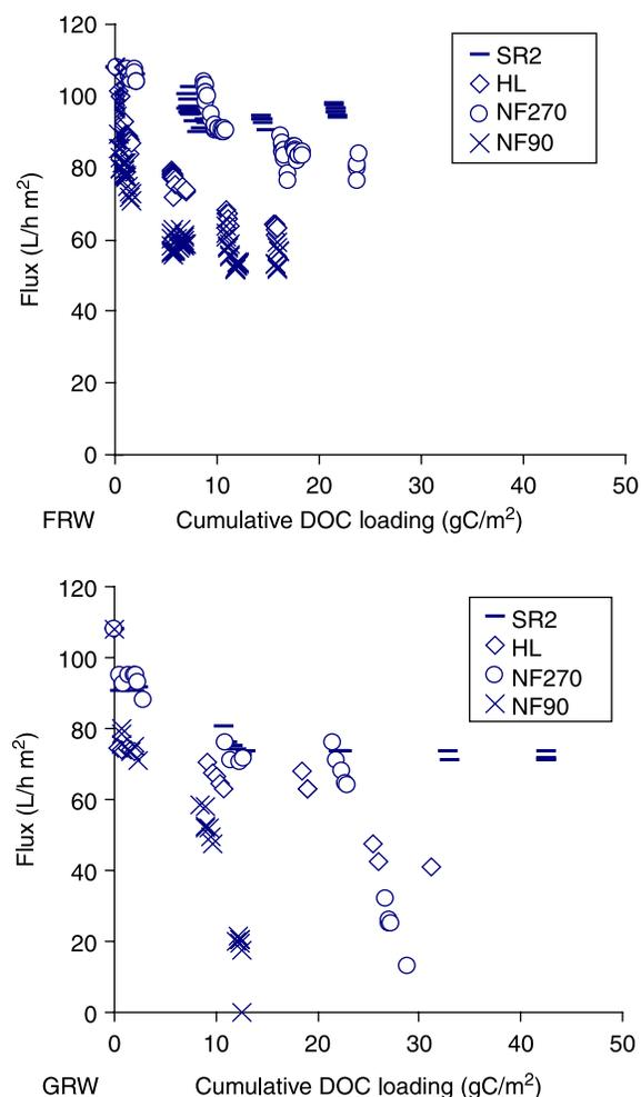
Figure 1 | Permeate flux versus cumulative DOC loading.
