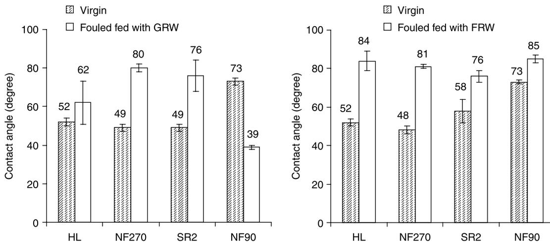
**Figure 6** | Contact angle of virgin and fouled membranes fed with GRW and FRW (data on left graph were determined using VCA2500 XE, those on right graph were determined using DSA 100S).
