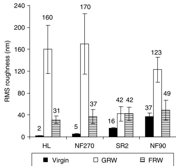
**Figure 5** | RMS roughness of virgin and fouled membranes fed with GRW and FRW.
