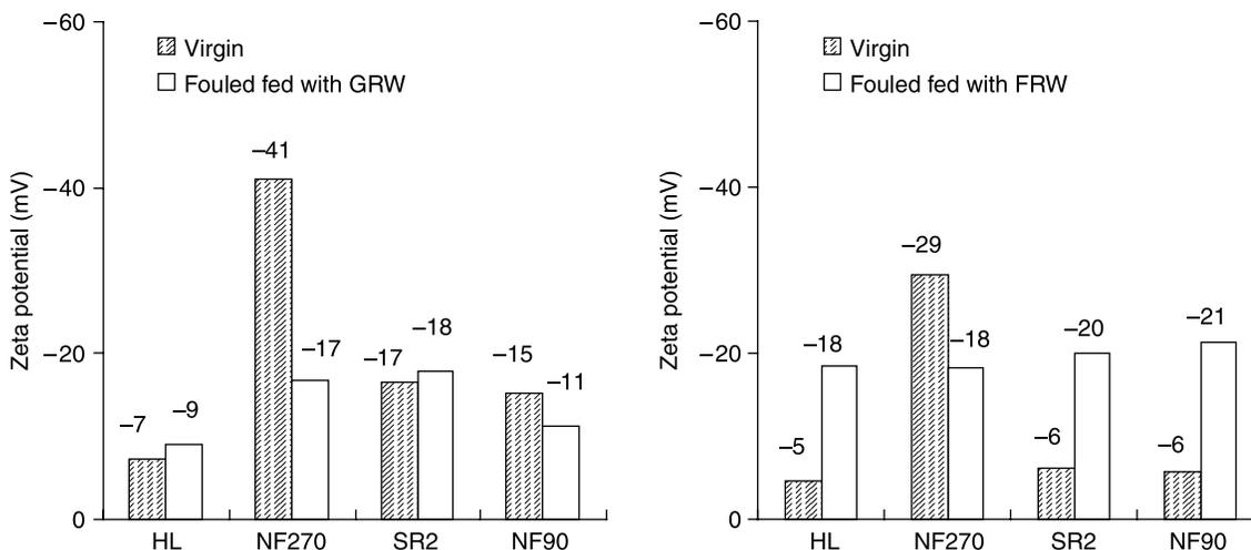
**Figure 7** | Zeta potential of virgin and fouled membranes fed with GRW and FRW (data on left graph were determined using EKA, those on right graph were determined using SurPASS).
