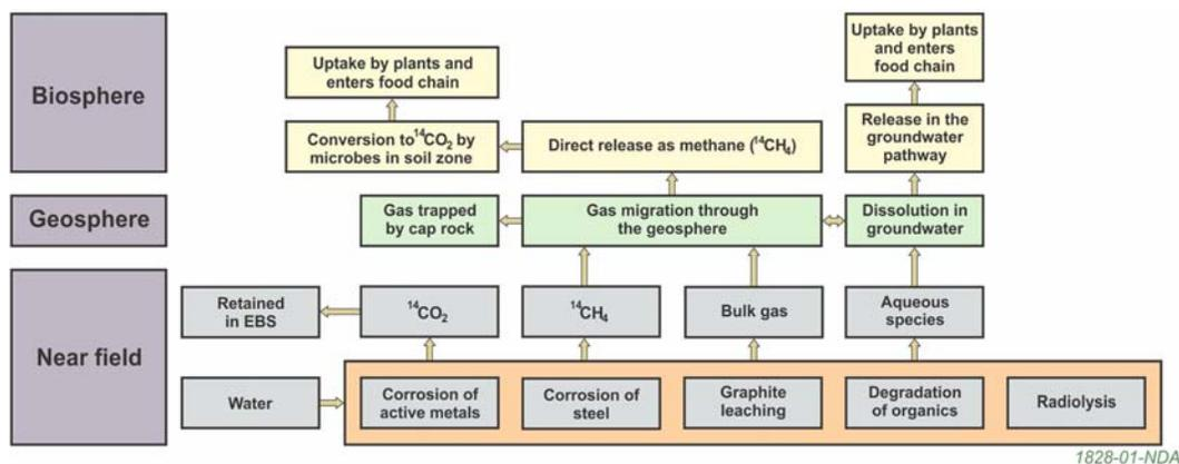
FIG. 1. The key processes for the generation and migration of  $^{14}\text{C}$ -bearing gases. Figure published with permission of the NDA.
