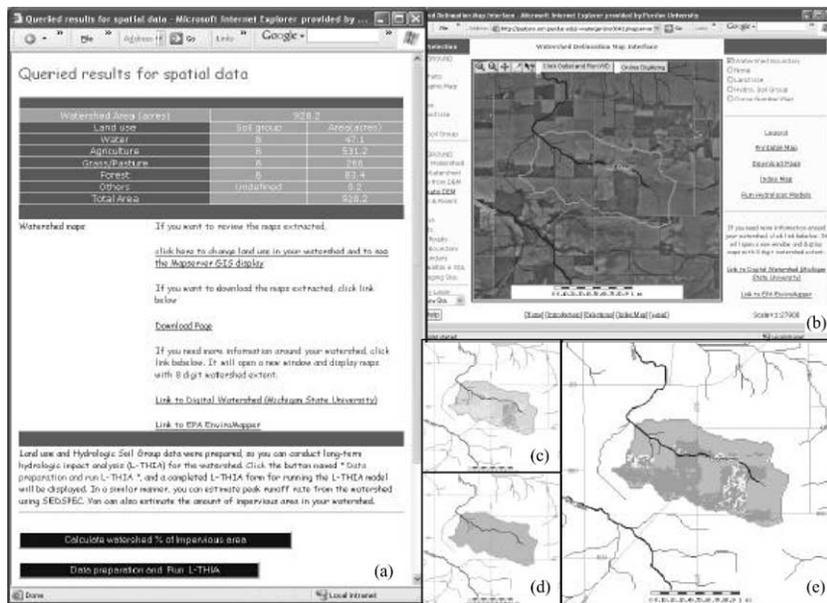
**Figure 4** | Web page for the delineated watershed output and results display. (a) Summarized watershed data tabulated with land use, hydrologic soil group and curve number. (b) Delineated watershed map display and map interface web page. (c) Land use map. (d) Hydrologic soil group map. (e) Curve number map.
