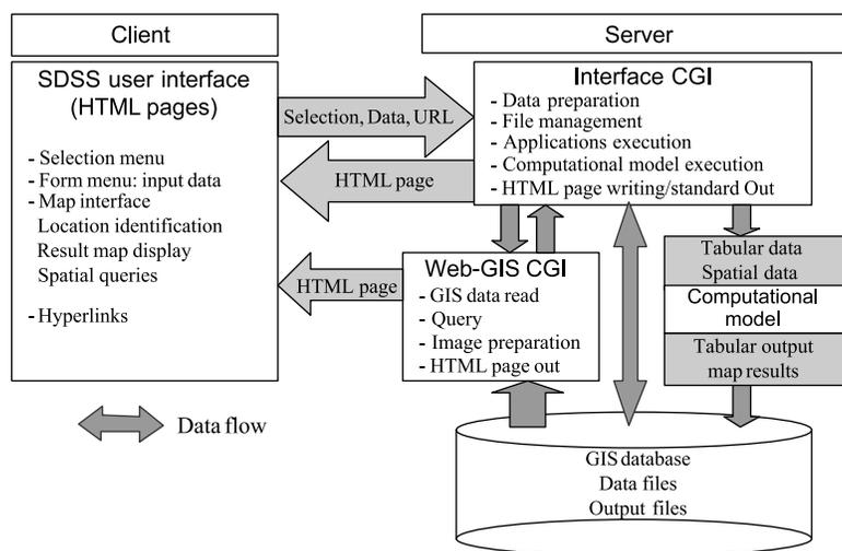
**Figure 1** | Schematic diagram for a web-based SDSS framework using common gateway interface.
