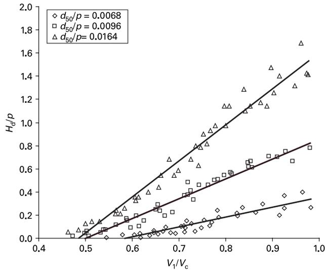
**Figure 11**  $H_d/p$  versus  $V_1/V_c$  with  $d_{50}/p$
