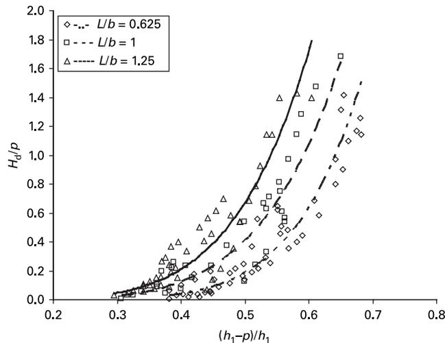
**Figure 10**  $H_d/p$  versus  $(h_1 - p)/h_1$  with  $L/b$
