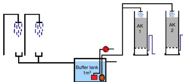
**Figure 2** | Schematic overview of the experimental pilot scale set-up.
