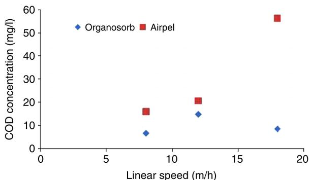
**Figure 4** | Effluent COD concentrations in the lab-scale tests as function of the linear speed in the column.
