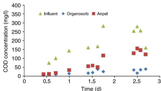
**Figure 6** | Influent and effluent COD concentrations during the experimental period.
