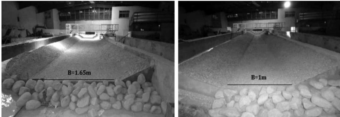
Figure 4 | The main channel with two different base widths.
