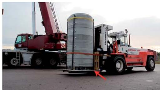
FIG. 3. A fully assembled distance block, the cable block can be seen at the bottom of the component (marked with a red arrow).
